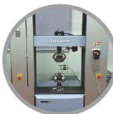
电子万能试验机 Electronic Universal Tester 测试抗拉强度、屈服强度、延伸率 To test tensile strength, yield strength and elongation
