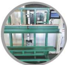
LED 数字测微仪 LED Digital Micrometer 金属带材宽度和侧弯测试 To measure strip width and camber
