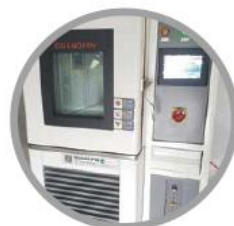
恒温恒湿试验箱 Temperature and Humidity Chamber 测试环境适应性 Test Environmental Adaptability
