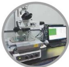
工具显微镜 Tool Microscope 观察与测量微观形貌 To observe and measure micro-morphology
